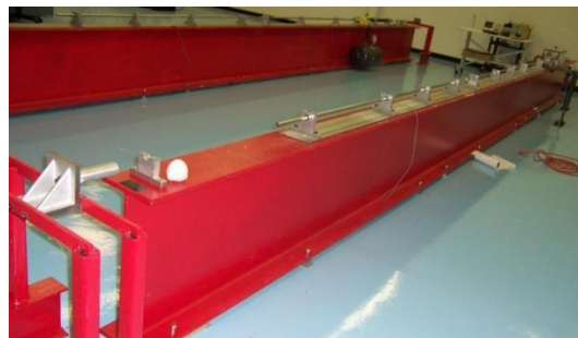
Figure 2. Hopkinson bar setup in the testing facility.
