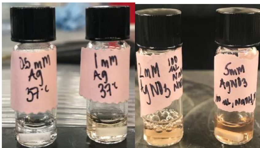
Figure 31. Ag Clusters at 37°C: The photo shows the color changes of the silver clusters made at 37°C. From left to right, the brown color increases in hue due to a higher silver concentration.
