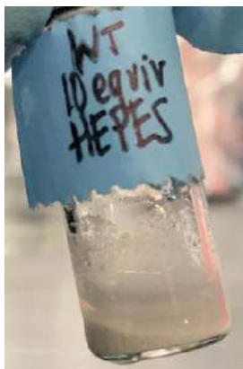
Figure 15. HEPES Buffer Precipitation: Image displaying the white precipitate that formed after 10 equivalents (5 \mu L) of 10M AgNO 3 was added to the solution with HEPES buffer and protein.
