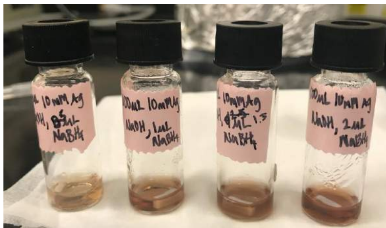
Figure 27. Increasing Amount of NaBH 4 : This image shows the different hues of brown created when different amounts of NaBH 4 was added to the solutions. From left the right, the amount of NaBH 4 increases in 0.5 μL increments.
