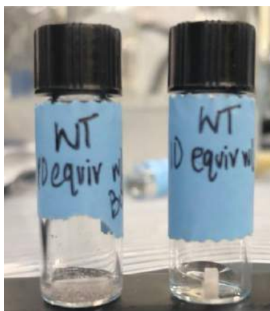
Figure 13. Buffer Versus Water: The vial on the left contains 10 equivalents of 10M silver and 95 \mu L of dialysis buffer that precipitated before protein was added to the mixture. The vial on the right contains 10 equivalents of silver and 95 \mu L of water.
