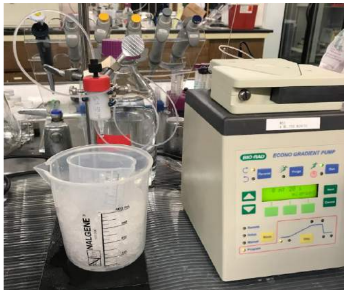
Figure 6. Strep-Trap Column Setup: This figure shows the Strep-Trap column setup and the Econo Gradient Pump machine which carries the protein to the column.
