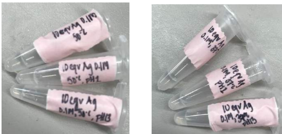
Figure 18. Ag Samples at Varying pH: Left image: 10 equivalents of 0.1M \text{AgNO}_3 at 50^\circ\text{C} with respect to pH 1, 7.8, and 13. Right image: 10 equivalents of 0.1M \text{AgNO}_3 at 37^\circ\text{C} with respect to pH 1, 7.8, and 13.
